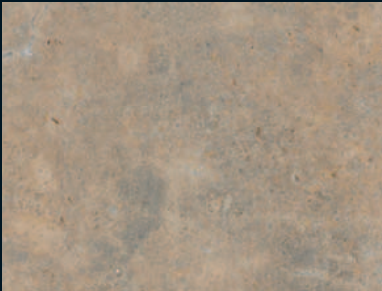
diageschliffen C30 diamond honed carborundum 30
