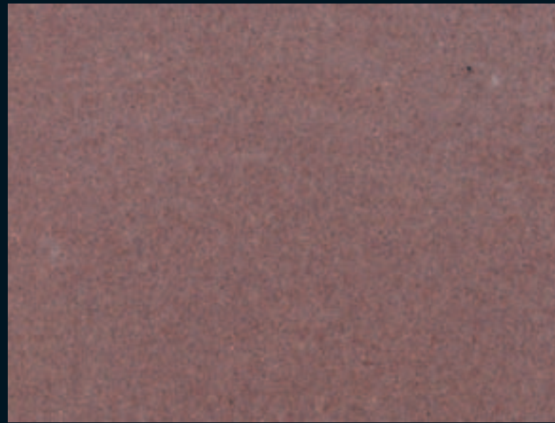
geschliffen C120 honed carborundum 120
